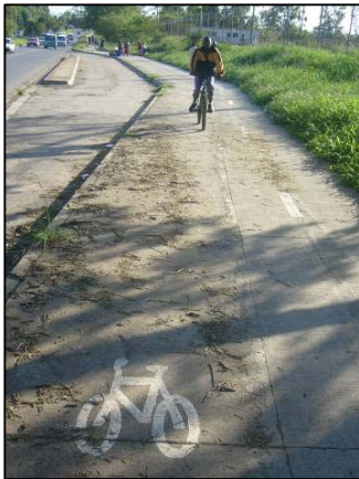
Path with markings for cyclists and line separating pedestrians and cyclists
